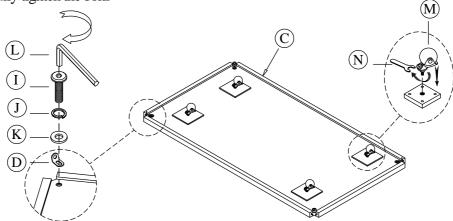
$Step \ 3: \ Using the \ Allen \ key \ to \ tighten \ all \ bolts$
